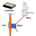
Figure 14: Ventilation Fan – Hydraulic.
