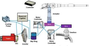
Figure 2: Gun Control – Electric.
