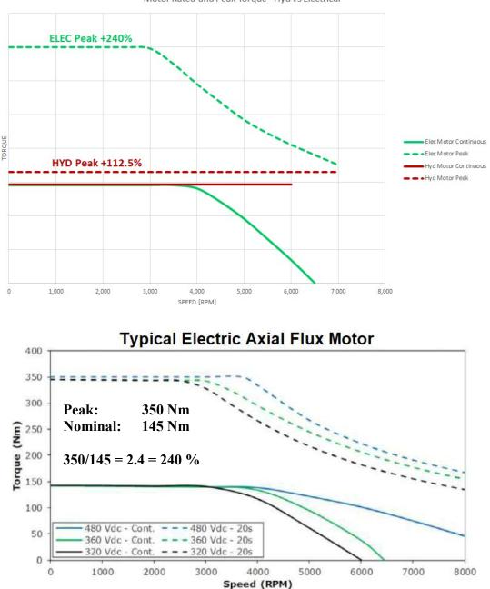
Motor Rated and Peak Torque - Hyd vs Electrical
