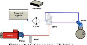
Figure 12: AC Compressor – Hydraulic.
