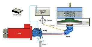
Figure 16: Cooling Fan – Hydraulic.
